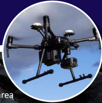
The spin-off operates in the environmental field, dealing with coastal area management, precision farming and contrasting coastal erosion. Thanks to SAPR (multirotor and fixed-wing drones, ENAC approved), equipped with special thermal sensors and laser scanners, photographic surveys are carried out in the visible, thermal or multi-spectral ranges, both on flat and vertical surfaces.
